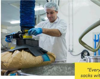
As a manufacturer of bakery ingredients, Bakels mix raw produce according to recipes by emptying sacks with ingredients into mixing tanks. Since they invested in TAWI vacuum lifters to help employees lift and empty heavy sacks, they have been able to keep a consistent and optimal production flow. With TAWI vacuum lifters the employees can handle several pallets of heavy sacks without straining their bodies or losing speed.
